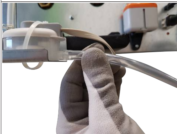
III. : 27: Raccorder le flexible d'aspiration
